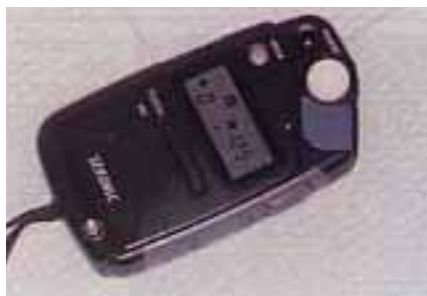
FIGURE 23. A typical incident light meter/flash meter used to determine exposure in many different types of lighting conditions, natural and artificial. For studio work, this will read the intensity of strobes and allow proper setting of cameras and lights.
