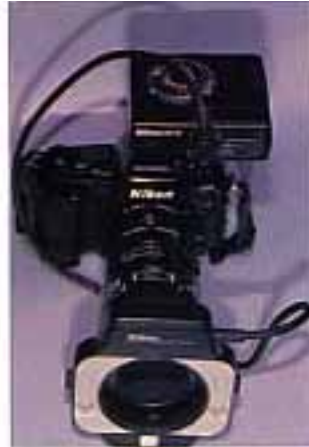
FIGURE 15. Dual-point source light with the light sources mounted at the front of the lens (Nikon 5B 29).
