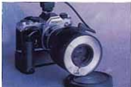
FIGURE 1. A typical dental clinical camera with a ring-light strobe surrounding the end of the lens. This is as close as a flash can get to the lens. Perfect for intraoral work, it is terrible for portraits. It is sure to produce red eye.
