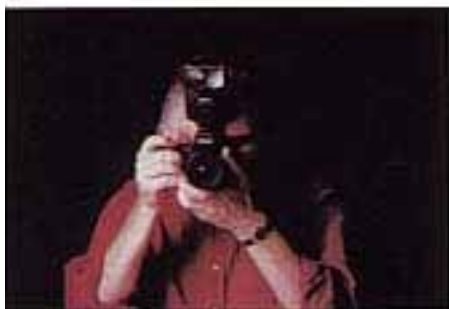
FIGURE 8. A standard 35 mm camera with a hot shoe-mounted flash on top of the camera. This is not enough separation of flash and lens and will still produce red eye.
