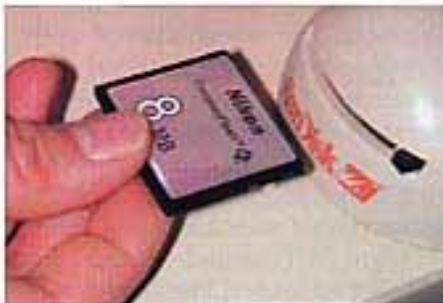
FIGURE 23. A "Compact Flash" solid state memory card is loaded into a card reader for downloading into a computer.
