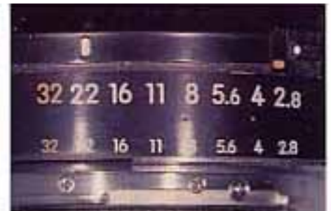
FIGURES 10. Aperture adjustment setting on the barrel of the lens. Changing the setting (f-stop) opens and closes the internal diaphragm of the lens, allowing in more or less light.
