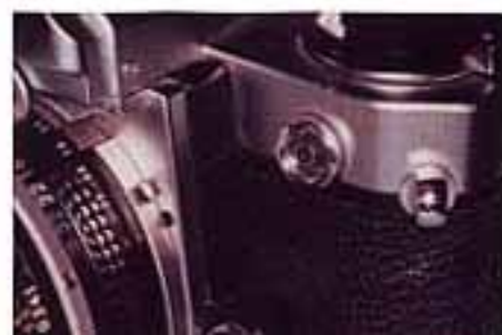
FIGURE 3. A PC connection found on cameras that will allow attachment of a PC cord to fire a remote strobe and deactivate the on-camera flash.
