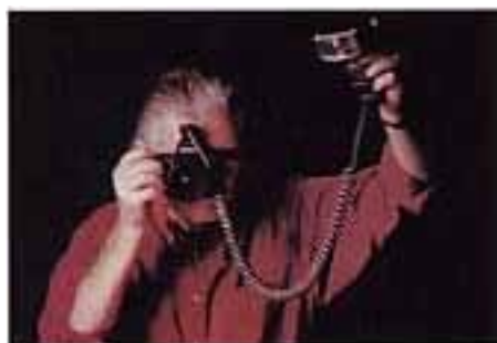
FIGURE 10. Same camera and flash as in Figure 8, but with an extension cord attached to the camera hot shoe and the flash. This enables the photographer to hold the flash in any position desired. In this case, 45 degrees to the side and 45 degrees above the subject will create Rembrandt lighting.
