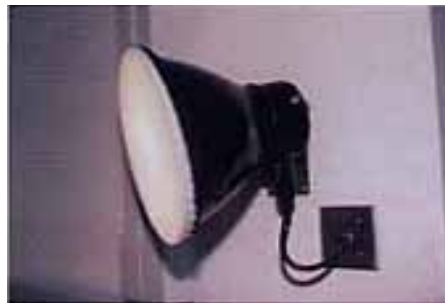
FIGURE 14. Permanently wall-mounted studio strobe with a cone-shaped reflector and white light diffuser over the end of the reflector.
