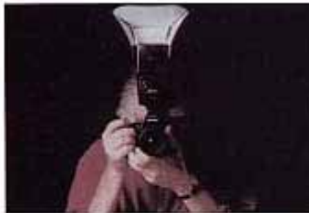
FIGURE 9. Same camera as Figure 8 but with flash positioned straight up and an extender and white reflector. This will eliminate red eye and give a softer, more diffuse light.
