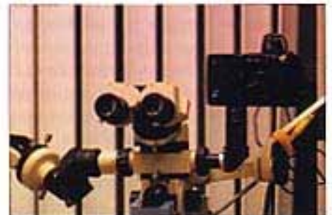
FIGURE 24. A microscope with a digital still camera (Nikon Coolpix 950) attached to a beam splitter. The display can be used to compose the photo, or better, output to a television visible to both patient and doctor. Power supply is by AC adapter cord directly into the camera so no batteries are necessary (photo courtesy of Gary Carr DDS).
