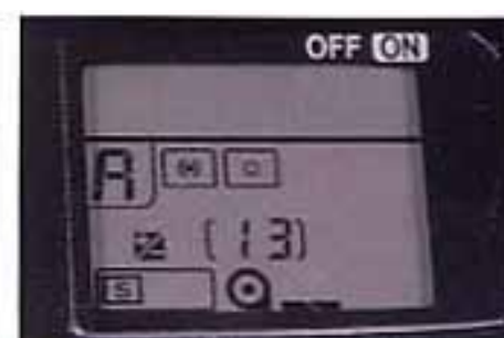
FIGURES 7 A, B, AND C. The aperture setting on some cameras will be a simple dial set to A or Ap as (a); or, in more sophisticated cameras, an exposure “mode” button (b) is pushed and the dial is adjusted until the LCD screen reads A or Ap (c).
