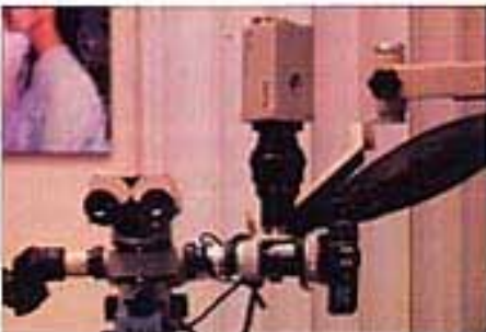
FIGURE 22. A microscope with a 35mm film camera and a video camera attached to the same side of a beam splitter (photo courtesy of Gary Carr, DDS).
